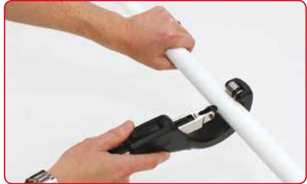
Use a set of Maincor disc type cutters for pipes larger than 32mm.
