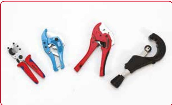
A range of cutter types are available to suit the pipe diameter.
