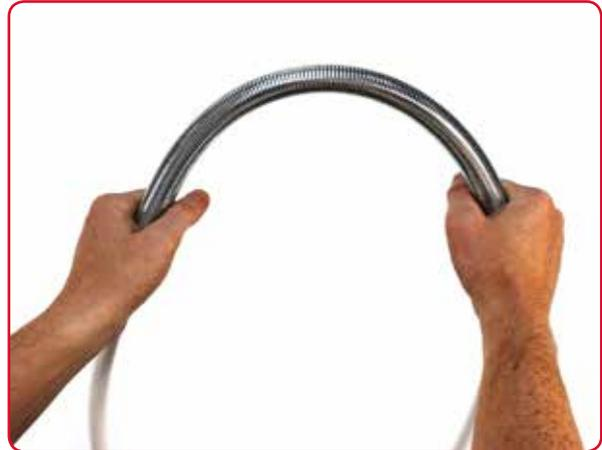
*Bending the pipe using an External Bending Spring.*
